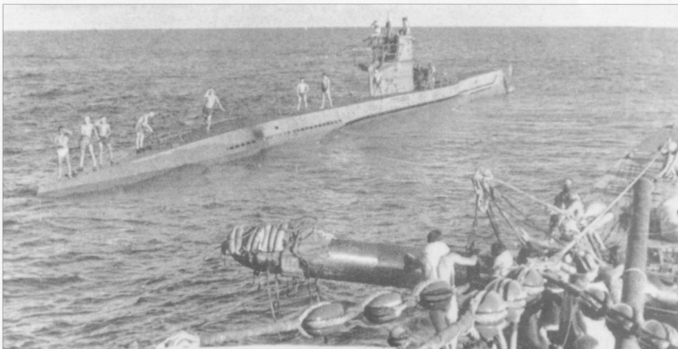
U 564 (Typ VII C) pobiera torpedy i paliwo od U 154 (Typ IX C), na zachód od archipelagu wysp Antyli, 07.1942. U 564 (Type VII C) taking on fuel and torpedoes from U 154 (Type IX C) west of the Antilles, July 1942.
